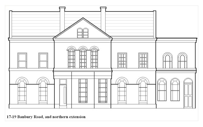
Figure 3. Line drawing of eastern elevation of 17-19 Banbury Road and its northern extension. Note that there are now lightwells and railings in front of 15 and 19.
