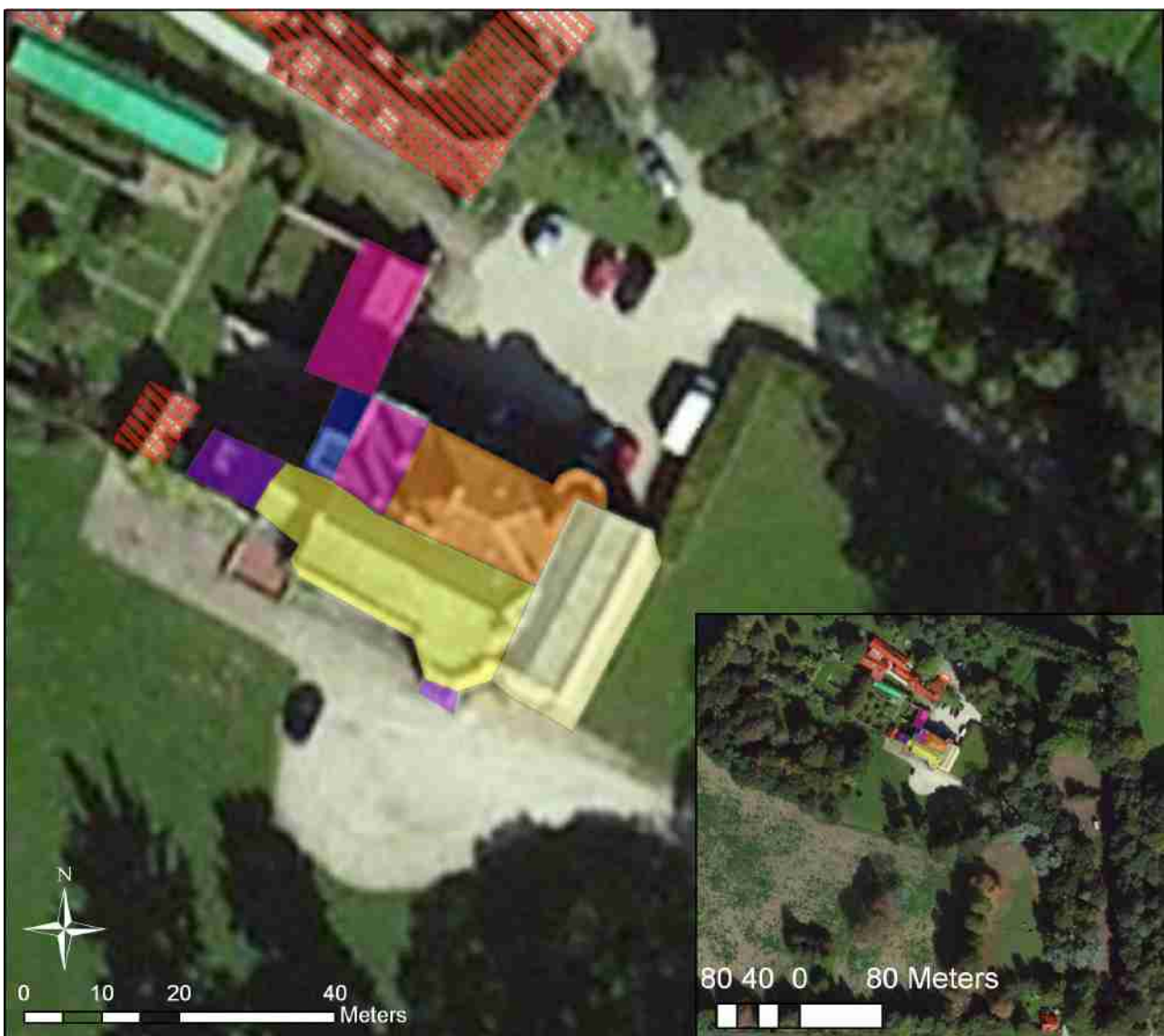
Figure 1. Tubney House and its outbuildings. The original c.1521 “Gollds” portion of the building is highlighted in cream. The 1811 extension is highlighted in yellow. The c.1840 extension is highlighted in orange. The c.1861 kitchen extension is highlighted in light purple. 20 th -century extensions are highlighted in purple. 21 st -century additions are highlighted in blue. The outbuildings are highlighted with red cross-hatching
