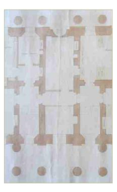
Figure 7 Changes to the first-floor transept. 7.1, left, extract from Smirke's 1831 plan. 7.2, centre, projected state of the space by 1901. 7.3, right, probable state of the space following 1901-2 alterations. All plans orientated with north at the bottom
